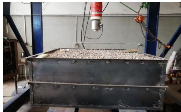
Fig. (11): The steel container filled with subbase layers.
