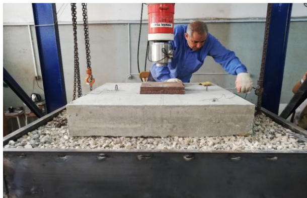
Fig. (12): The specimen was placed in the middle of container and the steel plate was placed in its center.
